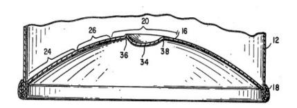
Concave closure element circumferentially joined to one end of the container side wall
