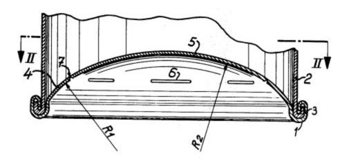
Outwardly concave bottom divided into an outer annular frusto-spherical part and a central dome by a plurality of tangential scores spaced apart in circular configuration
