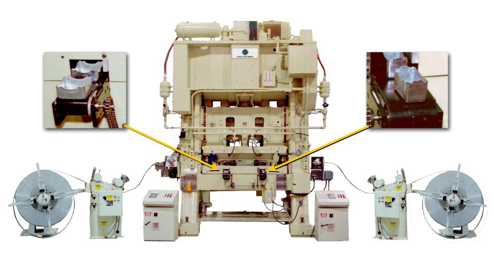
In draw/redraw canforming, a diameter reduction of 22% is possible per tooling pocket
