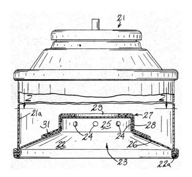
Under intense pressure, wall 22 will begin to bulge outwardly in a downward direction.
