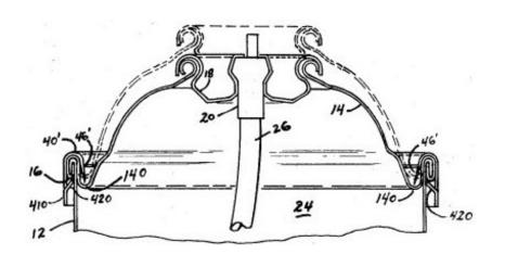
A dome venting cap, having a plurality of venting ports, is mounted exteriorly and directly located above the dimple
