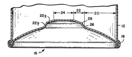
Concave annular outer area integrally joined to an inwardly protruding circular central area by annular intermediate area
