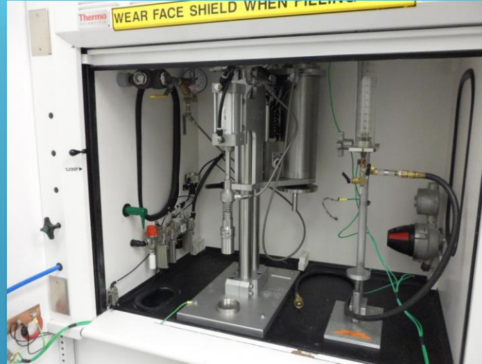
Benchtop Pneumatic TTV Gassing in vented Hood
