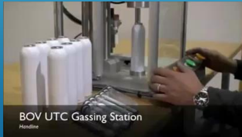
Benchtop Pneumatic TTV Gassing in vented Hood
