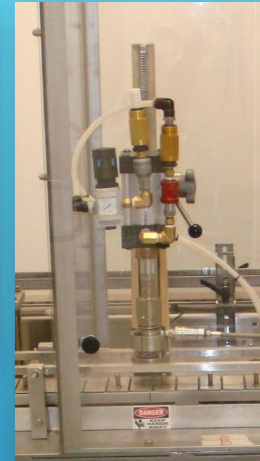
Single Head Through the Valve Gassing station
